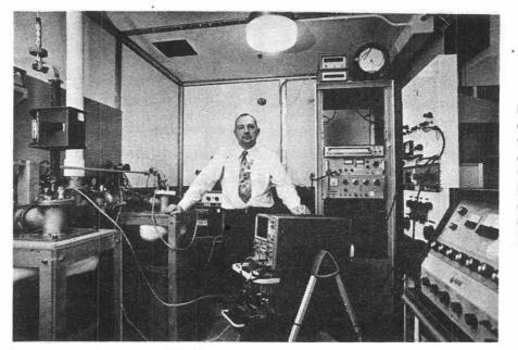
DAVE BRAUDAWAY (2552) developed this standard volt apparatus whose accuracy is comparable to that maintained by the National Bureau of Standards. Superconducting circuits and Josephson junctions were used.
